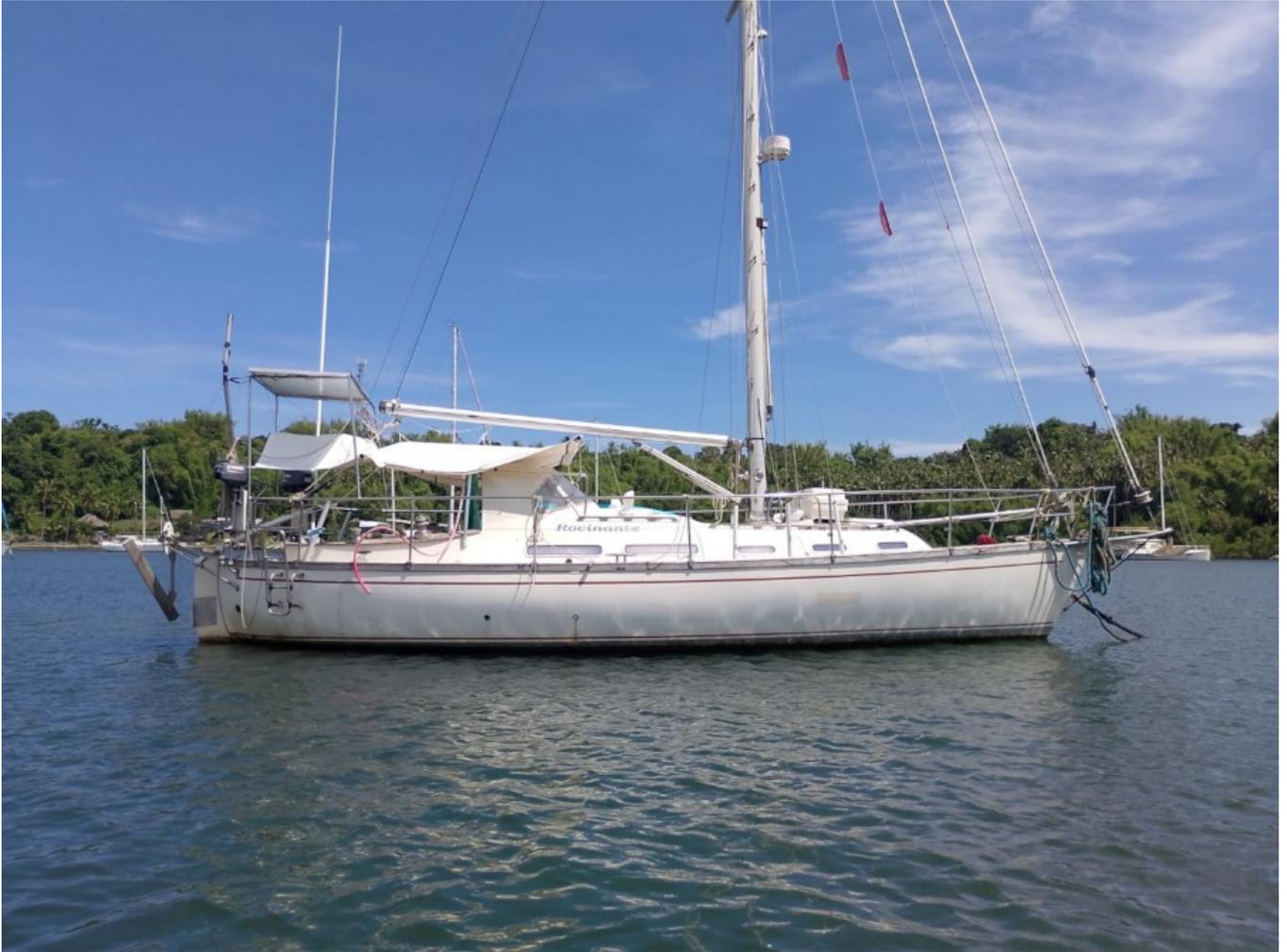
This world cruiser has full keel and is built of solid fiberglass. The boat has main sail with 2 reefs, double furling headsails and two whisker poles. The boat can be sailed downwind with the headsails opened on both sides, which gives easy control from cockpit.
